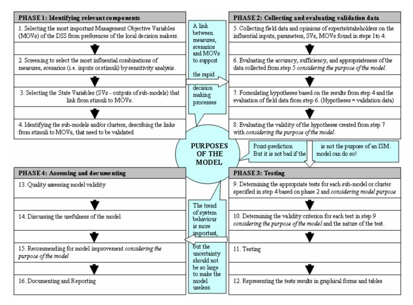
Figure 2.3. Flowchart for validation of ISMs
